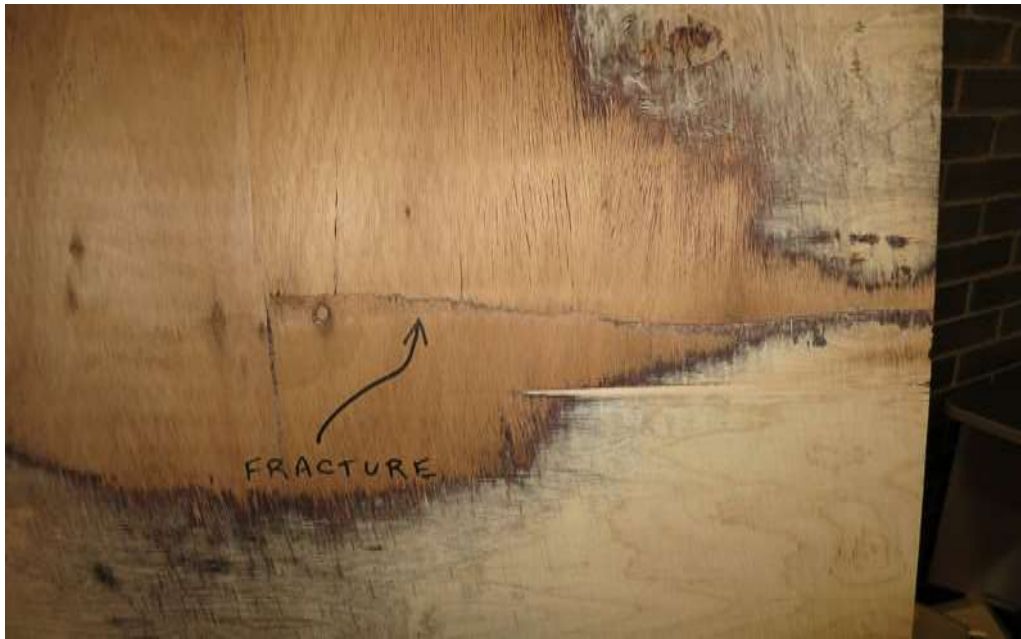
Figure 1. Imported plywood formwork that failed compliance tests against the Australian standard
