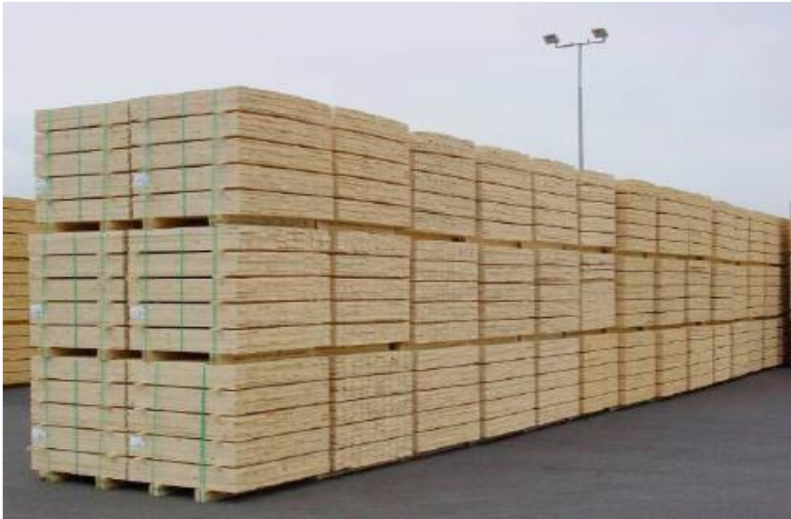
Figure 2: Avoid staggering or offsetting stacking of timber
