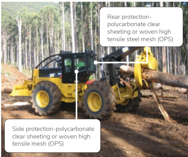
Figure 10: All wheeled drive skid steer skidder – side view
