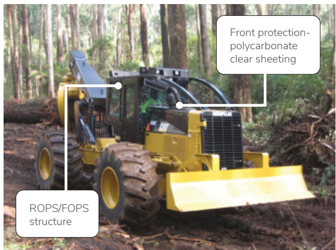
Figure 9: All wheeled drive skid steer skidder – front view
