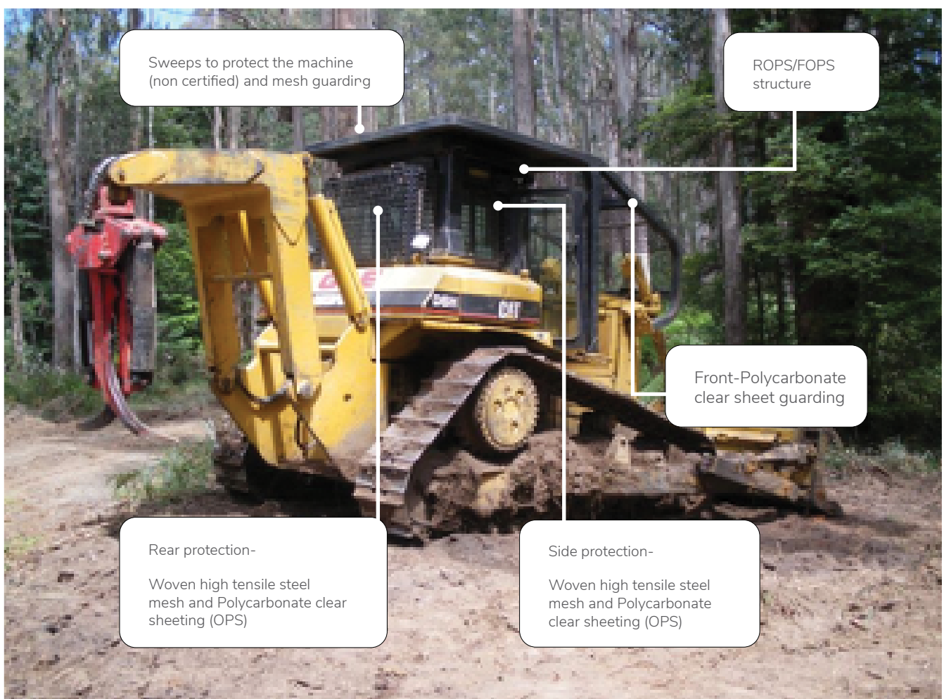
Figure 12: Crawler tractor fitted with snigging winch or log grapple
